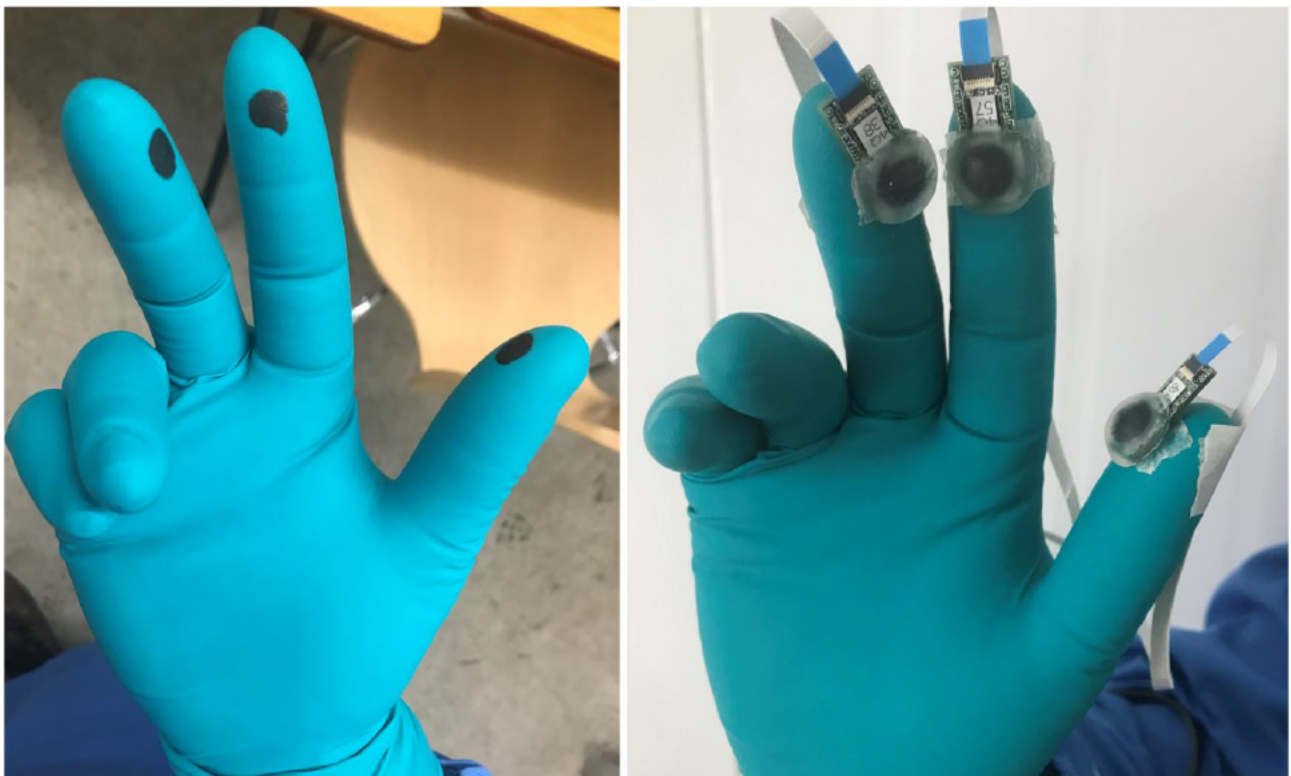
Figure 6 MITSUI sensors mounted on the expert picker gloves
