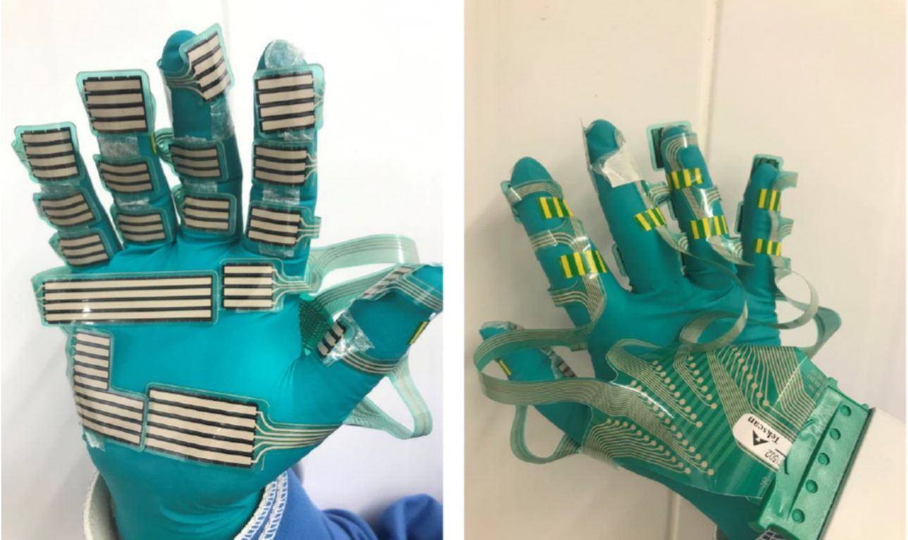
Figure 4 Tekscan Grip System sensing elements mounted on the mushroom picker's gloves
